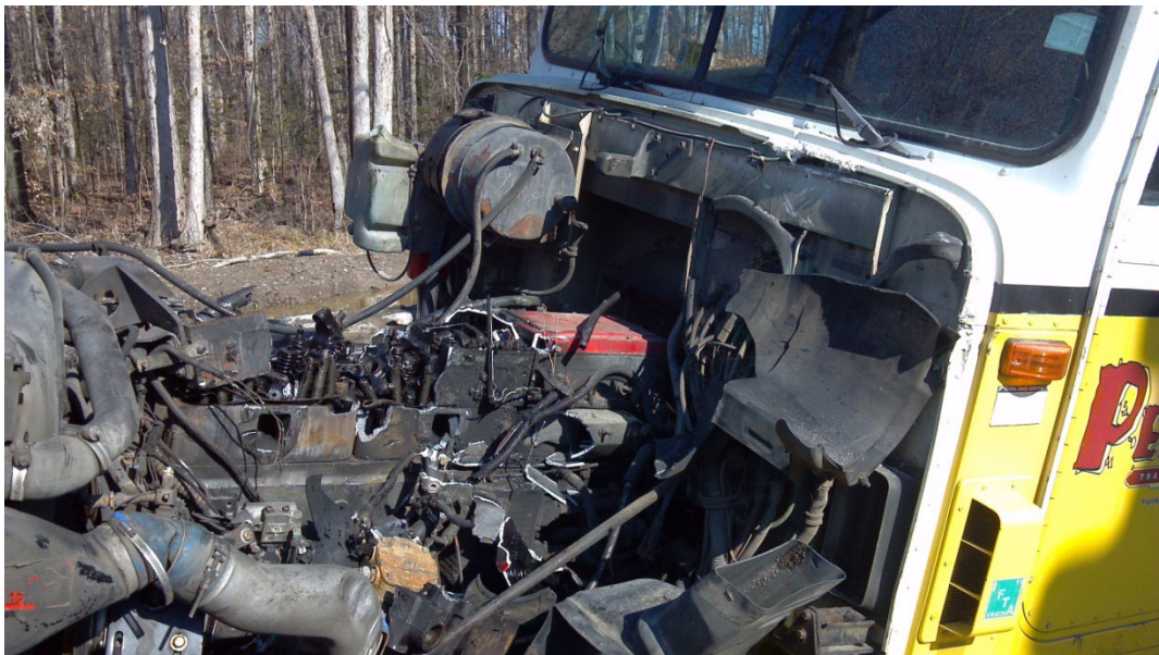
Example of visible destruction of the engine block
