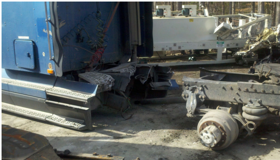
Example of chassis completely cut
