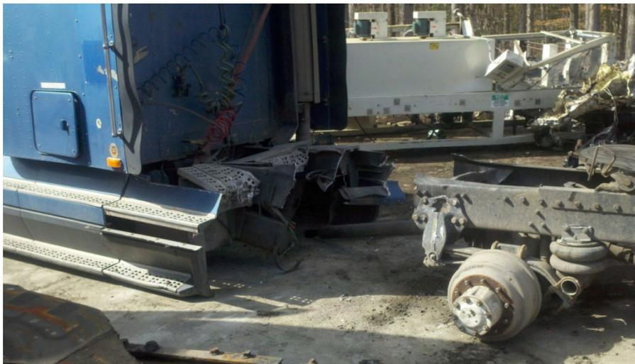
Example of chassis completely cut
