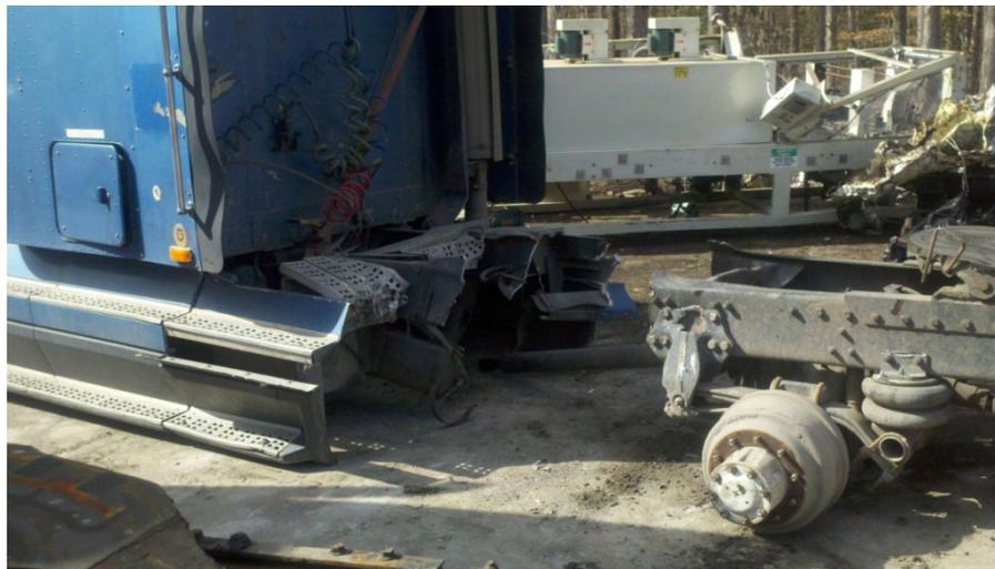
Example of chassis completely cut
