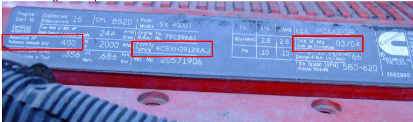
Cummins Nameplate: EPA Family Name – 4CEXH0912XAJ Engine Model Year - 2004 Engine Horsepower – 400 HP
