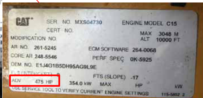
Caterpillar Nameplate (2 labels): EPA Family Name – 5CPXH0928EBK Engine Model Year - 2005 Engine Horsepower – 475 HP/1.0 02/08/2010
